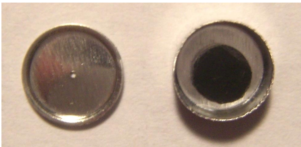
Figure 4.5. DSC Test Specimen Inside Open Aluminum Crucible with Lid.
