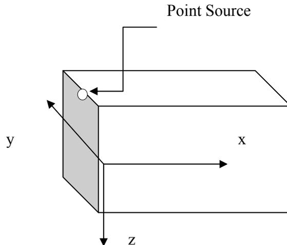
**Figure 3.1. Three-dimensional contaminant transport with an instantaneous input**
