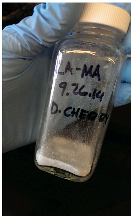
Figure 4.3 LA-MA Fatty Acid Eutectic Mixture at room temperature in a solid state.
