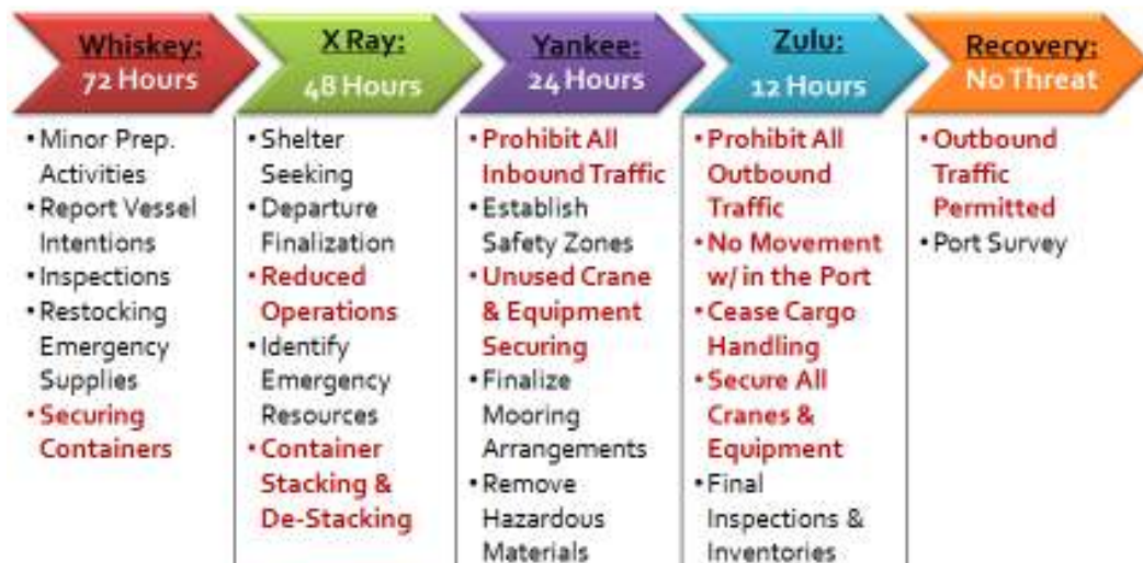
Figure 3.8. Port hurricane preparedness and response conditions and the associated procedures to be conducted
