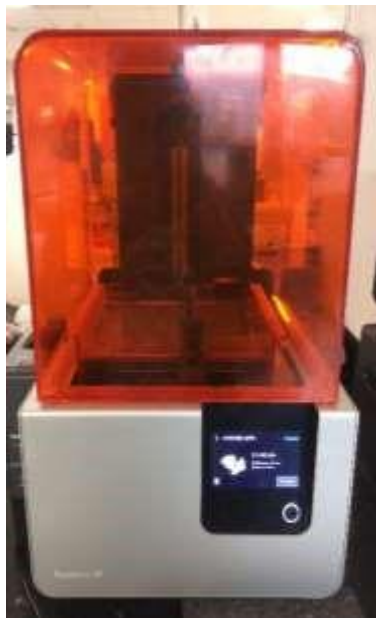
Figure 3.4: 3D Printer for preparing mold
