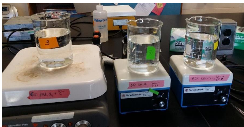
Figure 15. Experimental setup for kinetics release of sodium persulfate in water with agitation
