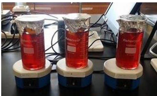
Figure 26. Kinetics release of potassium permanganate in water with agitation
