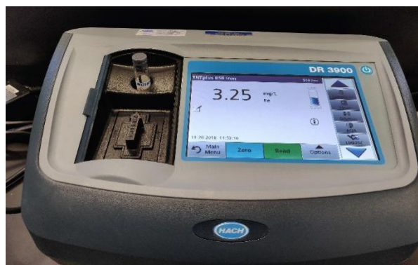
Figure 23. Identification of iron concentration in solution by bar-code determination method
