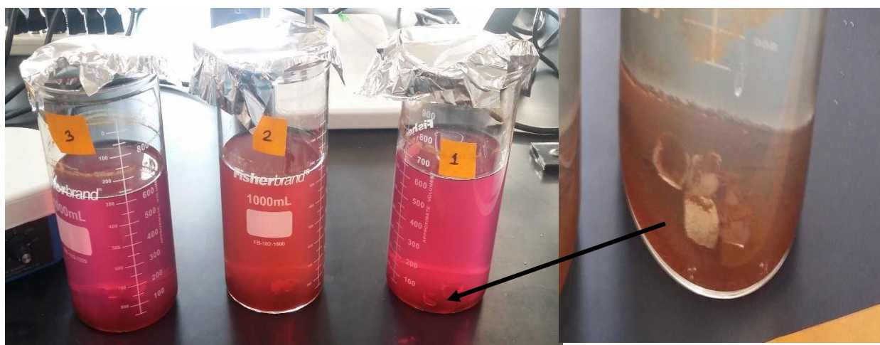
Figure 44. Accumulation of \text{MnO}_2 during kinetic release of \text{KMnO}_4 pellet
