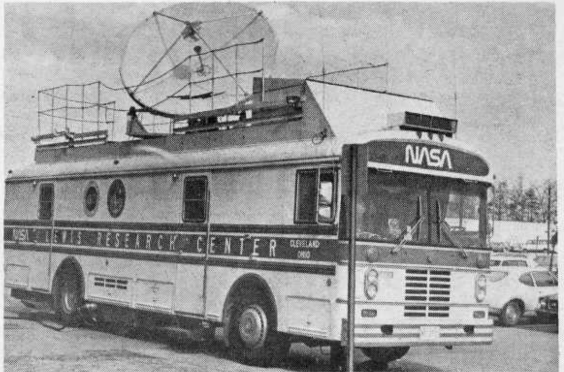
PET[Portable Earth Terminal], a 35-foot portable satellite communications terminal, will bounce off the Communication Technology Satellite. CTS is located 25,000 miles above the earth and transmits signals all over the world
